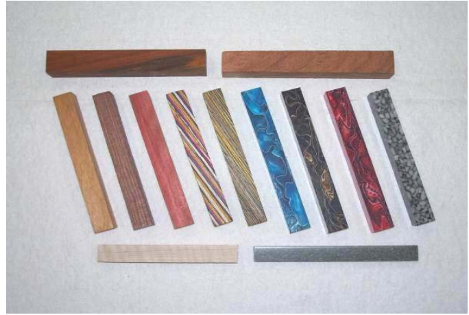
Exterior Selection: Barrels can be made from a variety of materials: ex: exotic woods, laminates & acrylics.
