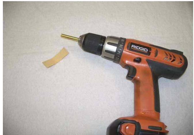
Preparing the tubes for gluing: Sand tube with 80 grit sandpaper. Lightly chucking tube in drill makes it easier!
