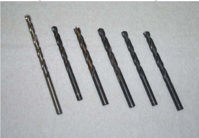
Drill bit selection: This also is determine by pen kit tubes. Brad point bits cut cleaner, but bullet points seem to wander less. Density and grain of barrel material may influence your decision.
