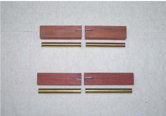
Sizing the blanks: Size & cut the blanks as dictated by pen kit tubes. Allow extra in case of drilling blow out. (1/16" extra on each end is sufficient)
