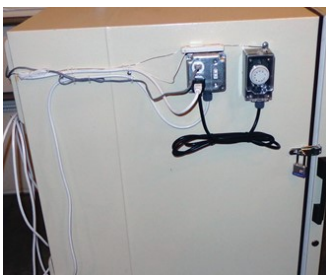
Mounted on the left hand side of the kiln are the controls, power switch and outlet as well as the greenhouse controller. Note the padlock for safety.
