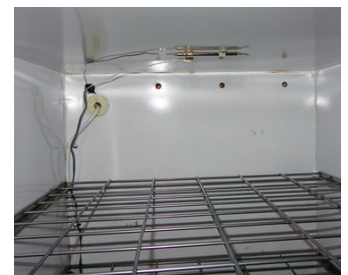
The sensor for the greenhouse controller is mounted to the ceiling inside of the kiln. The four holes drilled through the back wall of the freezer can be seen.
